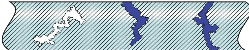
▶ Cast parts that are machined after impregnation can leak again if unfilled porosities are cut open.
